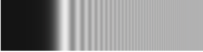
Fig. 4.28 Figure of diffraction from a half-plane screen. Simulation for an incident plane wave with \lambda = 1\mu\text{m} and an observation screen 10 cm away. The figure has dimensions 4 mm x 1 mm. Linear representation of intensity in the grayscale
